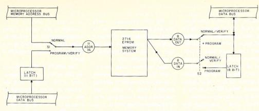
Fig. 1. A functional illustration of the isolation arrangement for address and data lines.
